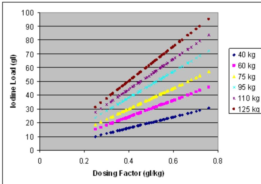
**Figure 9 - 3: Relationship Between Iodine Load and Weight Factor**
