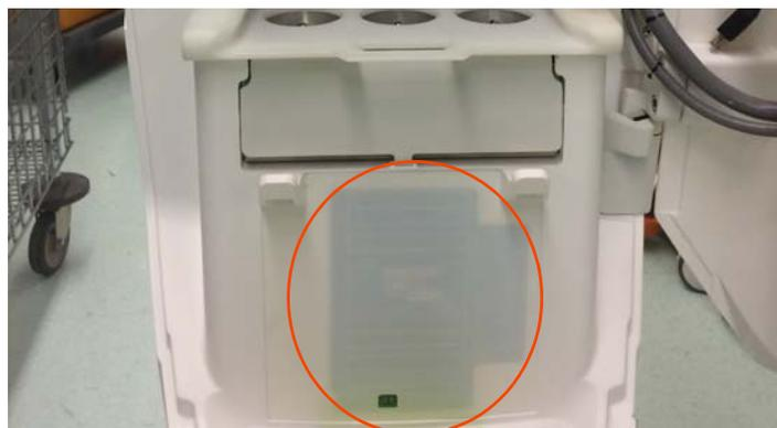
Figure 11 - 2: Prime Container Presence Sensor
